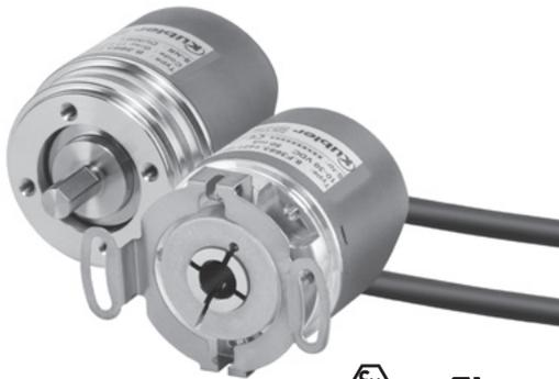
The Sendix F36 multiturn is an optical multiturn encoder in miniature format, without gears and with 100% insensitivity to magnetic fields. With a size of just 36 x 42 mm it offers a through hollow shaft of up to 8 mm or a blind hollow shaft of up to 10 mm.
